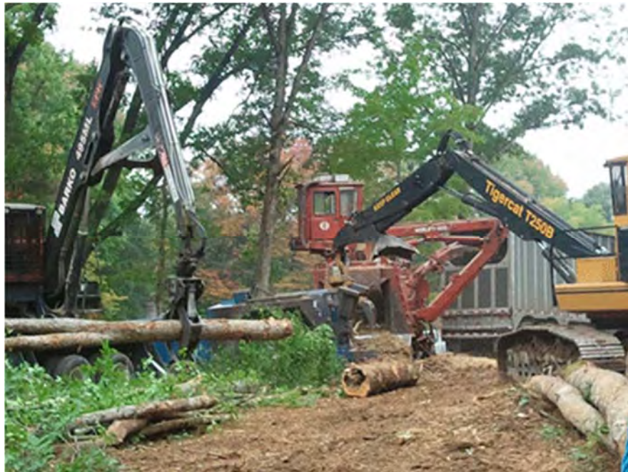
Combined sawlog and biomass harvesting operation sorting and processing materials for optimum utilization.
